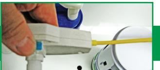
Push down the button on the handle switch box and insert the end of the spindle into the opening of the switch box. Make sure the square end of the spindle is inserted into the square at the back of the opening in the switch box. **NOTE:** Do not kink the yellow cable from the handle to the flush valve. The yellow cable needs to be in a sweeping curve.
