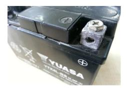
7. Use a socket wrench or pliers to loosen the screw of the battery lead, secure the un-terminated end into the hole of the primary battery positive (red/+) lead, as shown.
