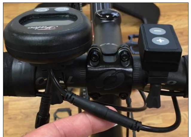
Figure 6: Connection between the console and the wireless plus minus buttons
