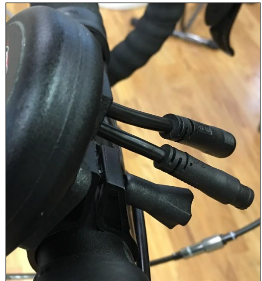
Figure 4: Console body mounted on the clamp and the tightening bolt
