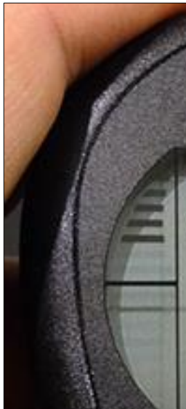
Figure 11: These bars on the top left-hand side of the console indicate the state of charge of the console when the motor is at stand-still. Six horizontal lines indicate the full state of charge.
