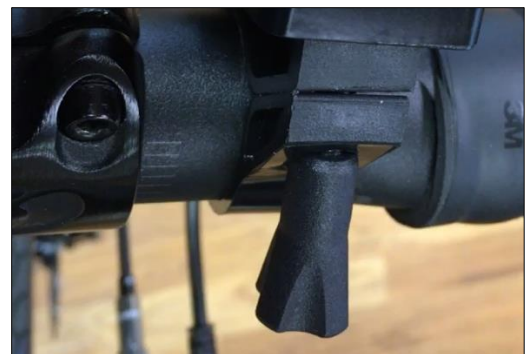
Figure 5: Mount the Wireless Plus Minus button in the same way as the console body
