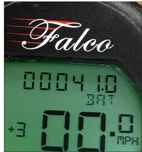
Figure 13: Once paired, the top line shows the battery voltage. Bottom left of this line shows the word, and to the bottom right shows the word BAT
