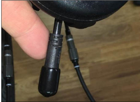
Figure 7: Junction box connector is not used in the wireless configuration. Please cover it with a cap or piece of tape to avoid dust or water penetration.
