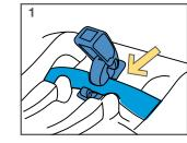
Pass the vehicle belt through the openings in the base labeled 'BELT PATH'
