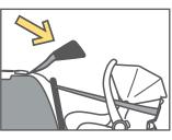
In some vehicles without a fixed parcel shelf an extension tether strap may be required. These are available in several different lengths and can be obtained from child restraint retail outlets.
