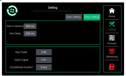
gas blow duration from laser on to beaming.
