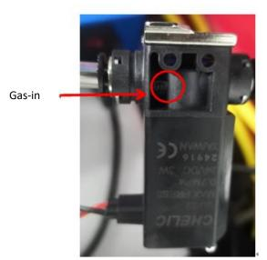
Gas valve ±: control switch of protective gas.
