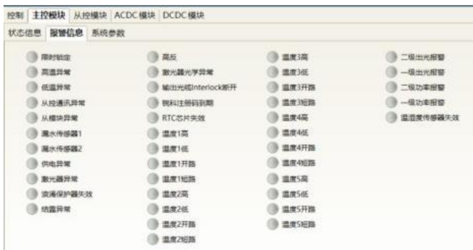
Figure 17 Alarm information interface of main control module
