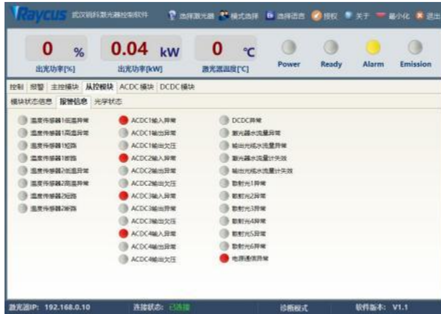
Figure 20 Slave control module alarm information interface
