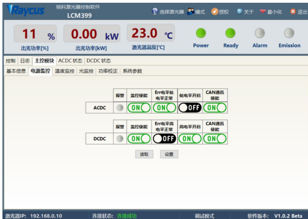
Figure 17 Alarm information interface of main control module
