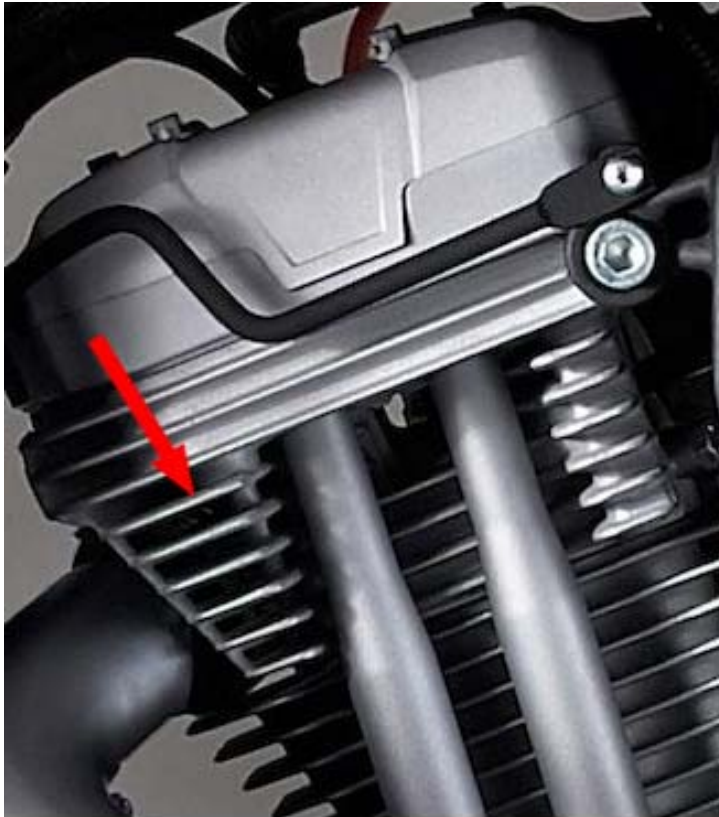
MOTORCYCLE ENGINE WITH COOLING FINS DESIGNED TO COOL OFF THE ENGINE
