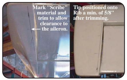
The tip is manufactured with additional "scribe" material which can be trimmed on installation to provide an accurate fit to the rib, allowing adequate clearance to the aileron.
