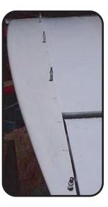
Once trimmed and drilled (#40 holes), Cleco tip into position at alternating holes and attach to rib with Recessed Truss-Head (Type A) #6 x 3/8" stainless self-tapping sheet metal screws and #6 Nylon Washers.
