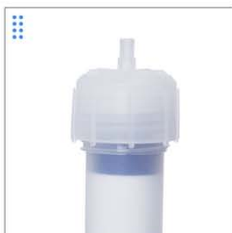
The tightening process will set the frit into place.
