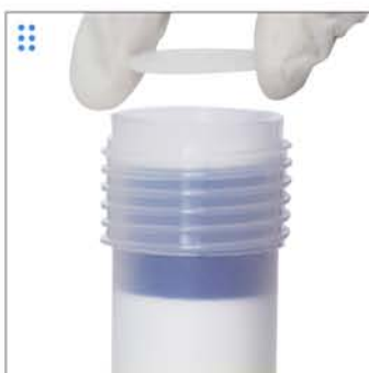
Add a dispersing unit on the top frit.
