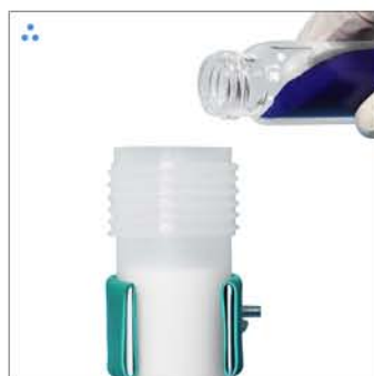
Add media into the headspace and tap lightly. Don't overfill.
