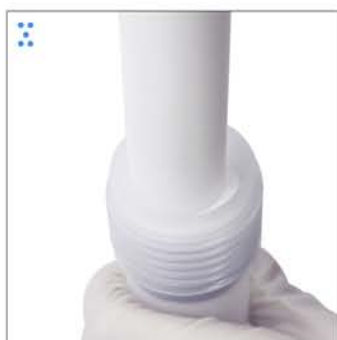
Use the frit insertion rod to press the fruit into space.
