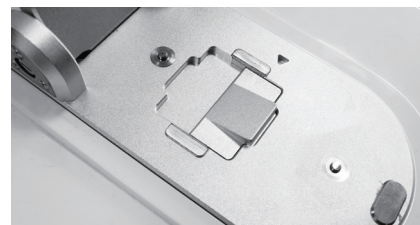
After the test is completed, wipe the measuring platform with dust-free paper to avoid sample residue
