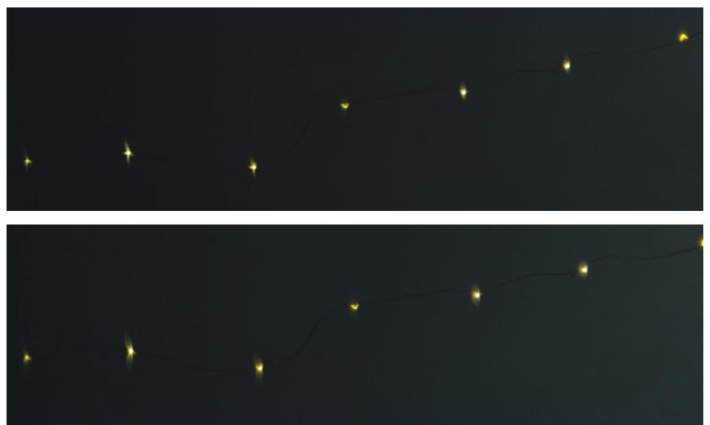
(TOP: Old Lens, BOTTOM: New Lens) Two images of Christmas-type lights at the edge of the frame at f/2.0 , to look at coma; edge is to the left as viewed. Both lenses are similar, and not that good. Past reviewers of the original lens have commented on the "healthy amount" of coma at f/2 (but gone by f/8 ), so the current findings are not really surprising.
