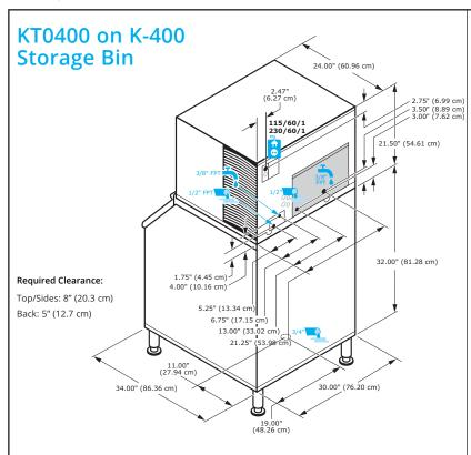
Water cooled condenser water usage/100 lbs. or 45.a Kg. of ice: 160 gals. / 606L.
