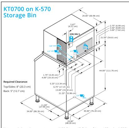
Water cooled condenser water usage/100 lbs. or 45.5 Kg. of ice: 160 gals. / 606L.
