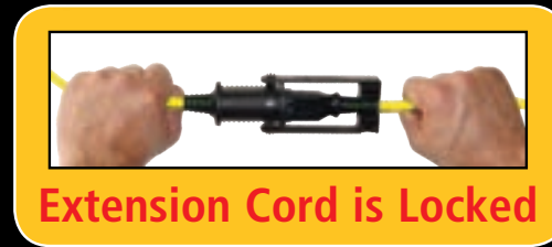
Close E-ZEE LOCK® latching mechanism onto the cable of the male plug. (Must attach to the cable, not the male plug)
