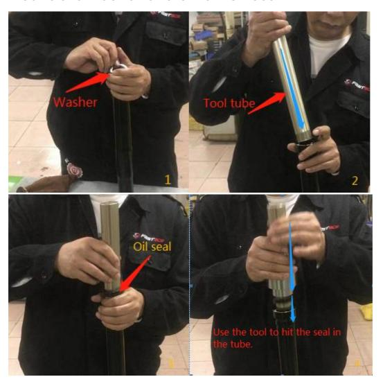
\*In figure 2: Use the tape to cover the thread to prevent to hurt the seals.
