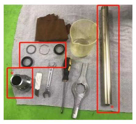
2. Loosen the top cap assembly from the outer tube.
