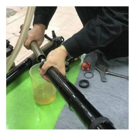
7. Remove the dust seal/ circlip/ oil seal/ washer.
