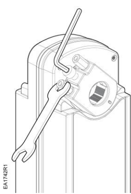
Figure 4. Fasten the Shaft Adapter to the Damper Shaft.
