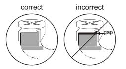
Fig.8. Correct / incorrect tightening of end limits
