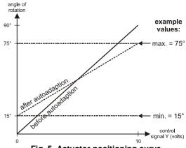
Fig. 5. Actuator positioning curve
