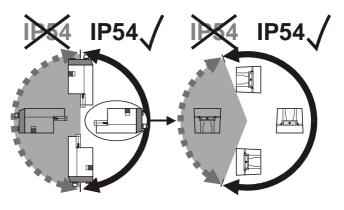
Fig. 9. Mounting for IP54
