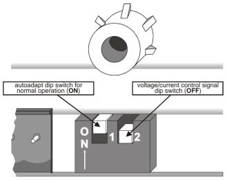
Fig. 4. Dip switches (view with PCB at bottom)
