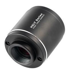
This camera uses a C-Mount standard lens mount. The camera can be mounted directly to a microscope which provides a C-Mount photo port, or it can be mounted to an ocular or photo port by using an optional compensating lens. The C-Mount standard uses a 1" (25.4mm) diameter with 32TPI (0.794mm pitch).
