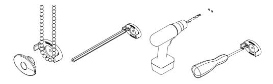
Re-assemble the cord tidy with the chain and fix it in previously marked position with a screw through the centre hole.
