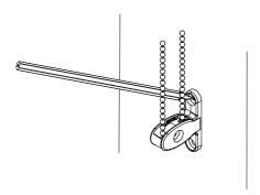
Mark the remaining hole position before drilling and plugging both location holes if necessary.
