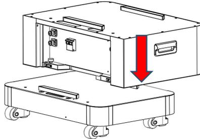
Place the battery module at the assembly position on base in the direction of arrow
