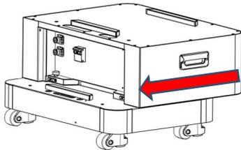
Step 3: Align the transverse locating pin at the bottom of battery box with the axis of transverse locating hole of base. push the battery to the extent that the longitudinal locating pin of battery is aligned with the longitudinal locating hole of base, put down the longitudinal locating pin at the back of battery, and complete the installation after the clamping sound of pin.
