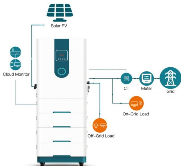
The system can be used in off-grid system and grid-connected system, and is suitable for many applications such as home users, small agriculture, small business and electric vehicle charging.
