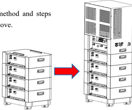
Step 6: Fix the equipment, and after completing all installations and debugging, apply the rear cover of battery box, install two fixing supports on the back of inverter, punch two expansion screws on the wall according to the height of screw holes of the fixing support, move the equipment against the wall, and lock the fixing support on the expansion screw.
