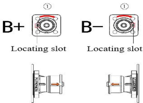
The power line plug has two locating pins. Align the plug with the socket arrow, insert the power line plug into the socket, and complete the connection when a crisp sound is heard.
