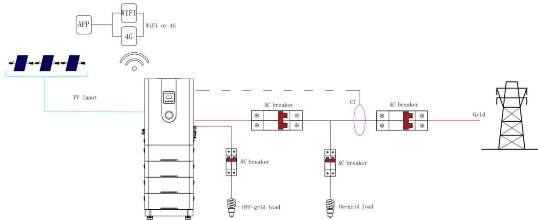
Instruction: the above picture is a single-line schematic diagram which is applicable to three-phase systems.
