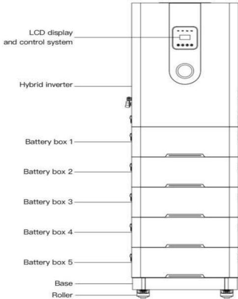
Instruction: Lenercom LC-E2 8-12kW products can accommodate up to 7 battery modules for three-phase model. In case of more than 6 battery modules, please contact your dealer or Lenercom. We will recommend the installation method according to the actual situation of the site
