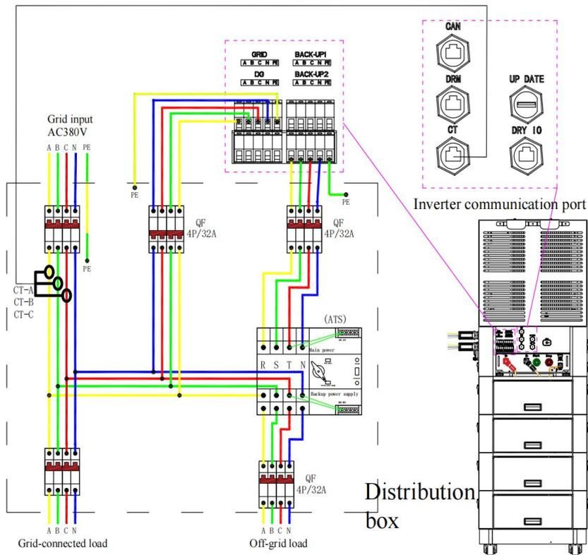
2. Wiring diagram without dual power switch (three-phase models):
