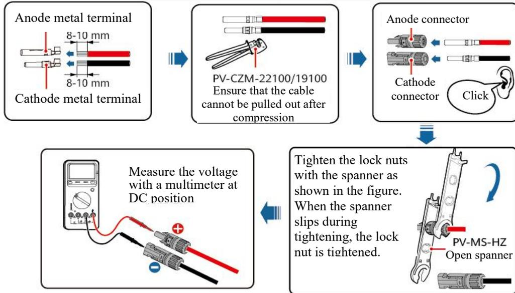
Use Staubli MC4 anode, cathode metal terminals and DC connectors. The use of other incompatible models of anode, cathode metal terminals and DC connectors may result in serious consequences, and the resulting equipment damage is not covered by the warranty.
