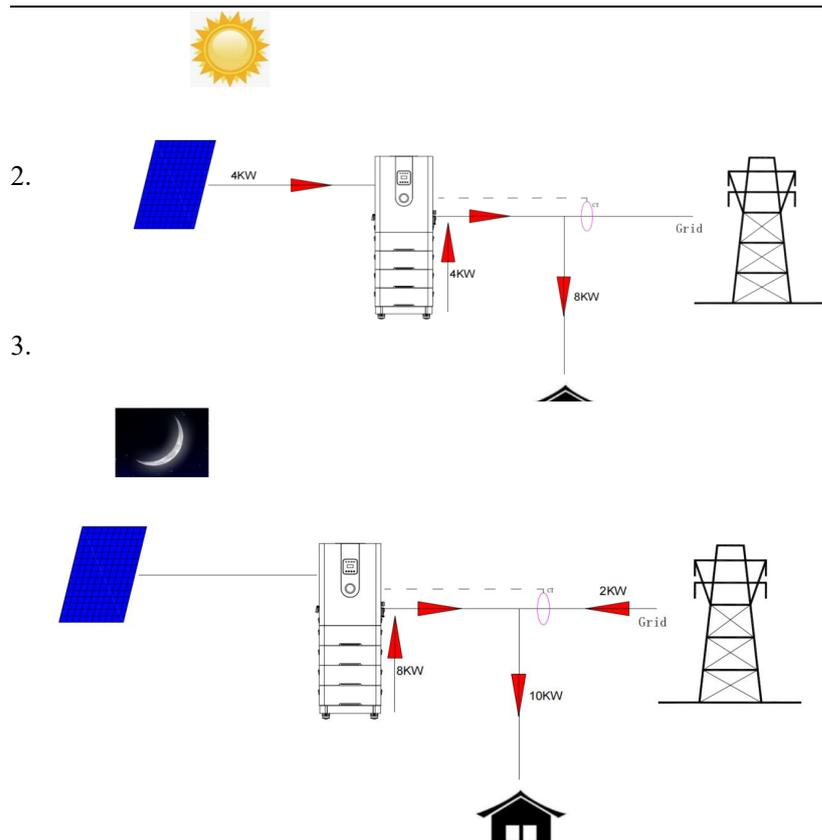
**Working mode: Self-generating and self-use, surplus electricity fed to grid**
