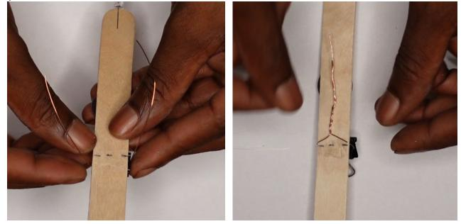
Step 8: Take the other piece of the copper tap and place it over the short side (cathode) of the LED as well as the twisted wire.
