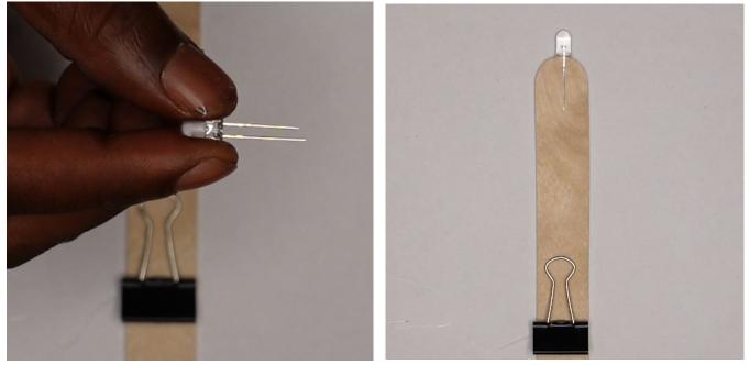
Step 4: Take one piece of your copper tape and place it on the end of your popsicle stick, making sure you cover the end of the LED anode. Fold the copper take back onto itself just under the binder clip.
