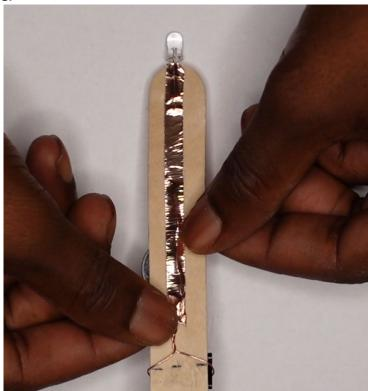
Step 9: Flip down the binder clip leg to close the circuit and illuminate your LED.
