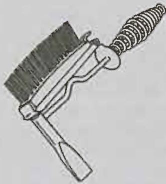
Spring Handle Chipping Hammer with Wire Brush on top
