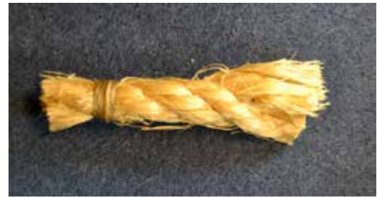
This natural fiber cordage is three-stranded and right laid. Each strand has many fibers.
