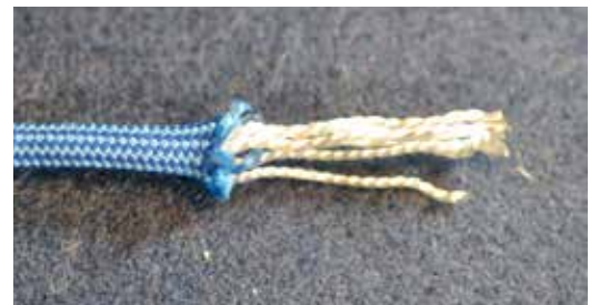
Paracord is made with a braided sheath and a core of twisted strands.
