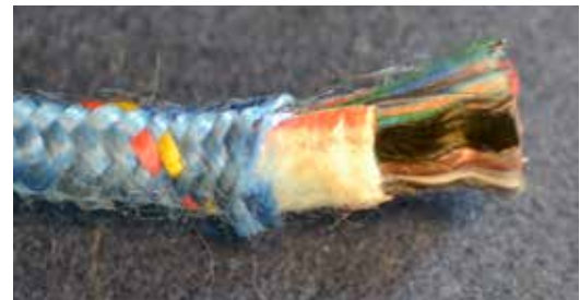
This synthetic sheath and core rope has an outer sheath, an inside paper core, and an inner core of individual fibers.
