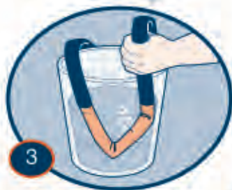
3 Locate the leak and then patch it.
