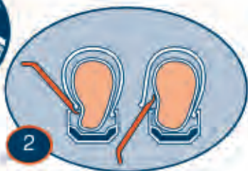
2 This view shows a cross-section of the tire, tube and tire lever.
