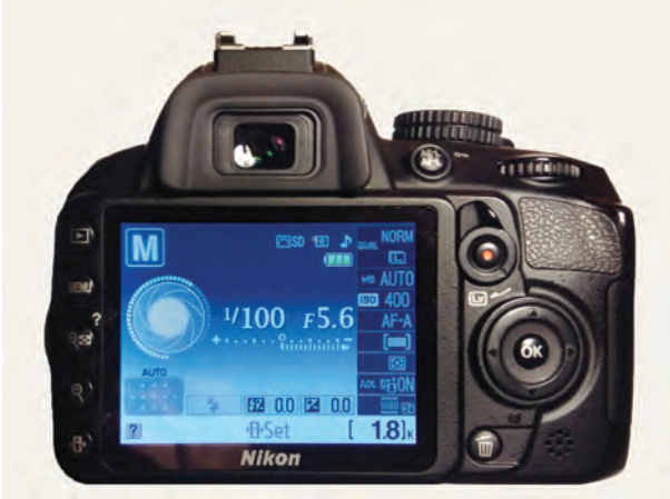
The screen on this 25LR indicates an exposure of 1/100 second at f5.6
