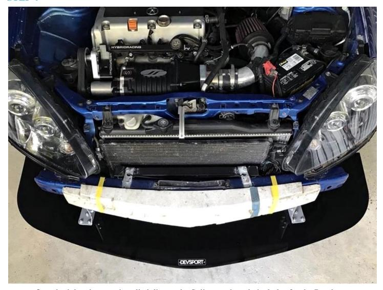
Once both brackets are installed, lineup the Splitter and mark the holes for the Brackets. Drill the holes in the Splitter and mount the Splitter to the Brackets using the 8mm hex bolts.
