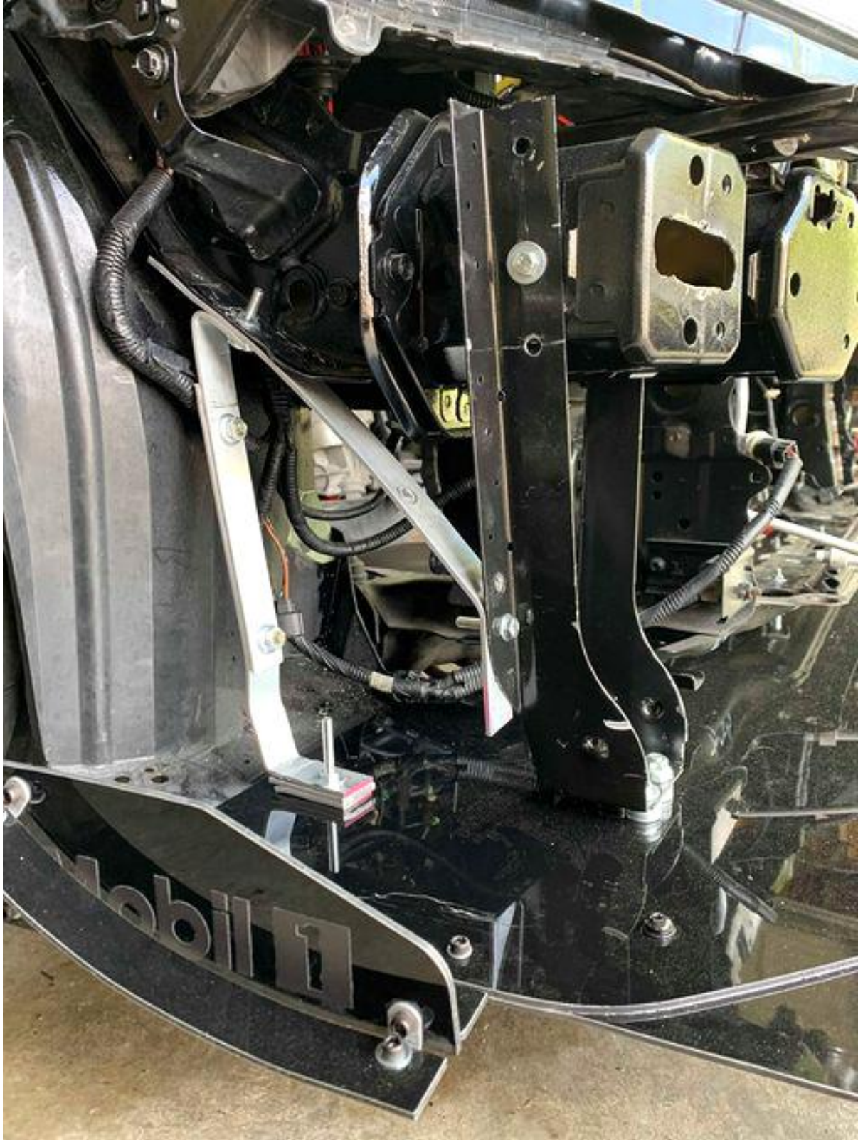
Custom brackets supporting the side section of the Splitter via the bumper crash beam support rail.
