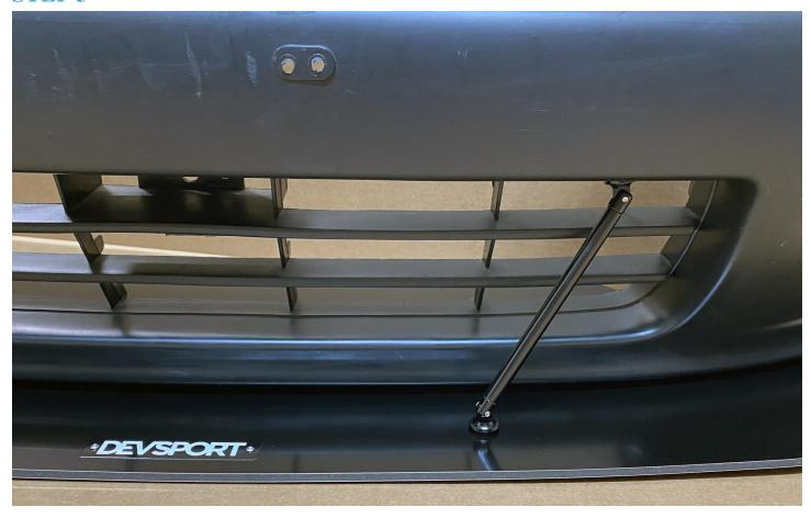
Install Support Rods in a vertical position. Tighten all nuts once Support Rod in finally position.
