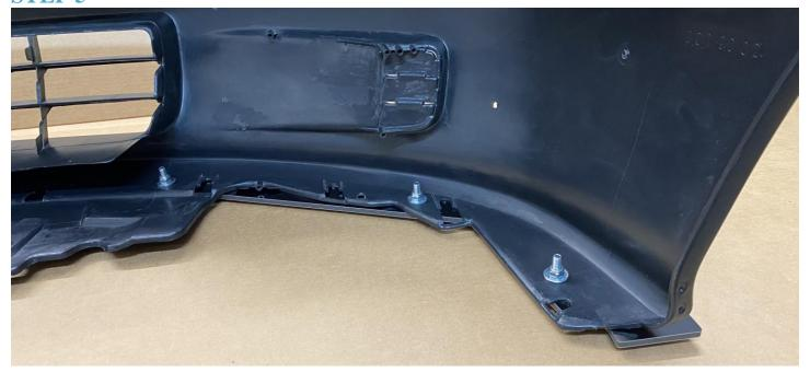
Once all holes are drilled into the bumper, re-align the Splitter to the bumper. Insert the bolts through each hole and tighten the nuts. (Thread lock highly recommended)
