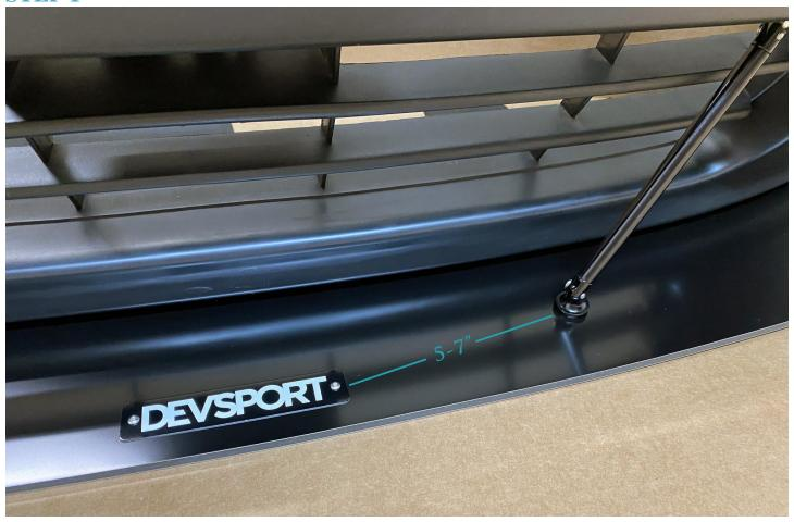
When spacing the Support Rods, the standard distance is 5-7" from the badge on each side.
