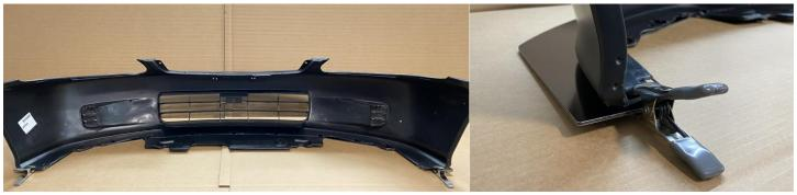
Remove the front bumper and align the Splitter to the bumper. Clamp down each side.
