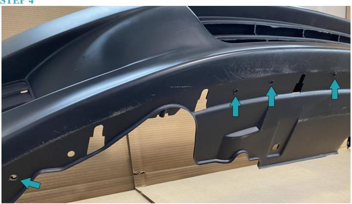
Drill bolt holes into the bumper using a 3/8" drill bit.
