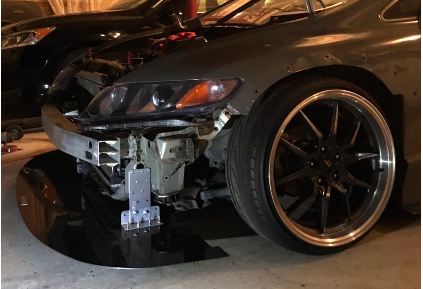
Custom brackets supporting the side sections of the Splitter via the radiator support.
