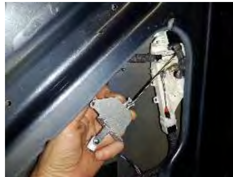
Disconnect inner door handle cable Figure 2.
