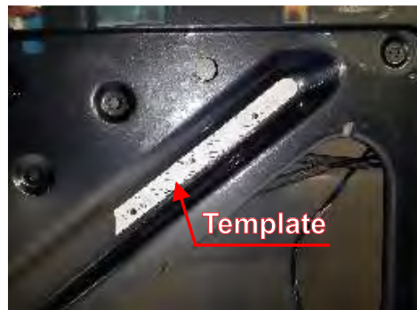
Drill 6.5 mm two holes Figure 4.
