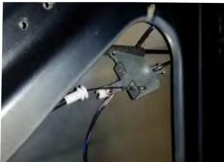
Connect inner door handle cable to the new position Figure 3.
