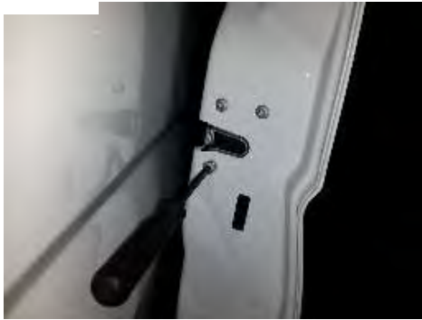
Pull off door latch mechanism Figure 1.
