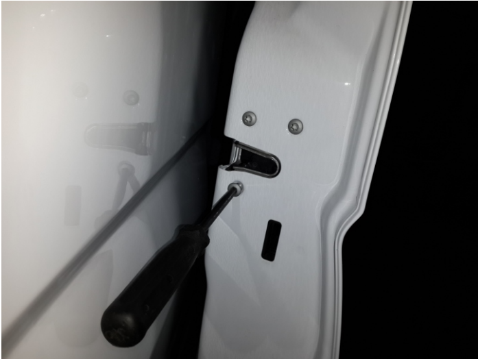
Figure 1. Pull off door latch mechanism
