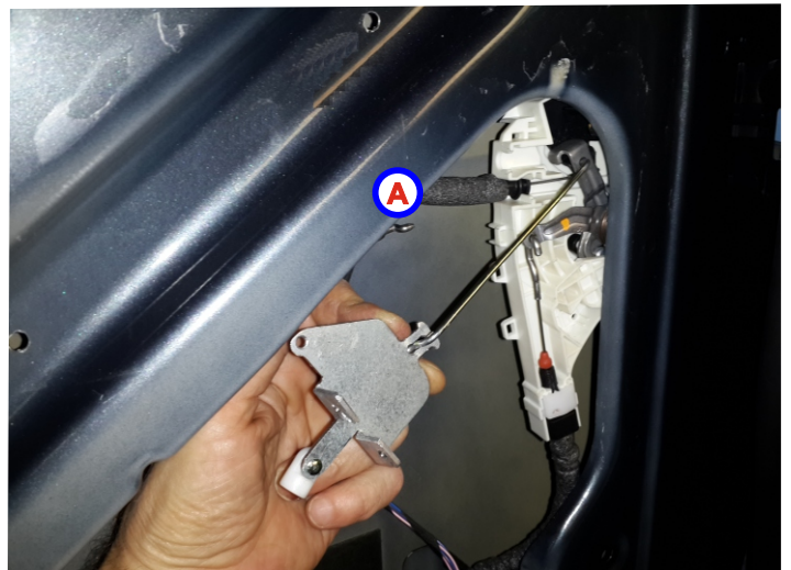
Figure 2. Disconnect inner door handle cable (A)
