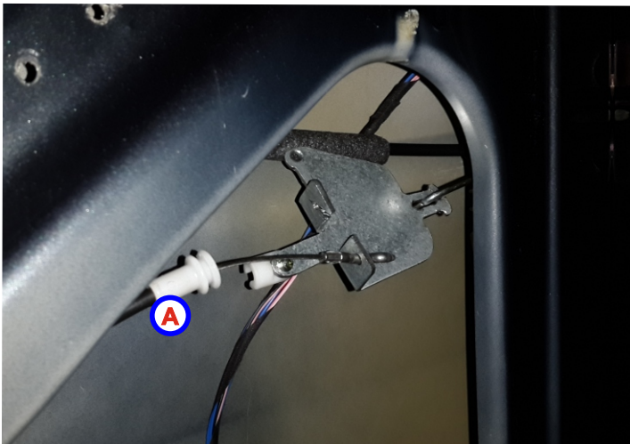
Figure 3. Connect inner door handle cable to the new position
