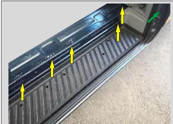
Figure 1. Remove original step
