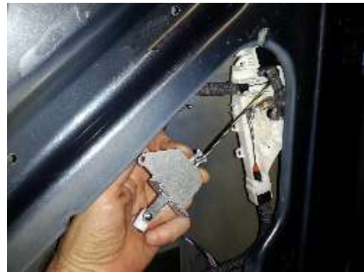
Disconnect inner door handle cable Figure 2.
