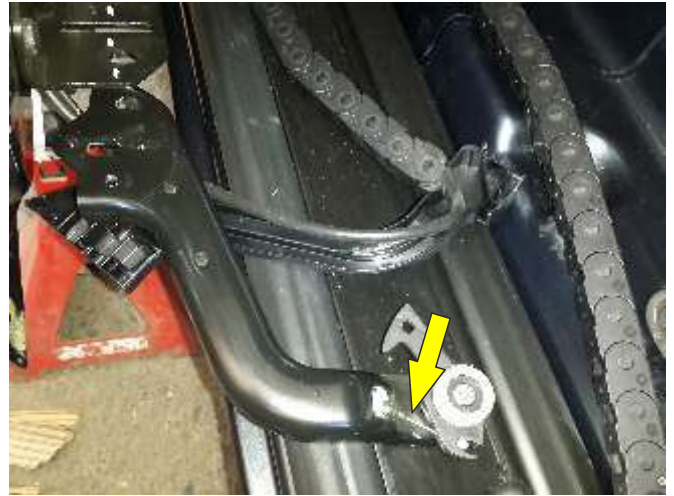
Disconnect the cable and move him to a new location
