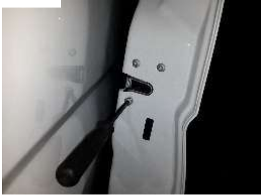
Pull off door latch mechanism Figure 1.
