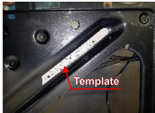
Drill 6.5 mm two holes Figure 4.
