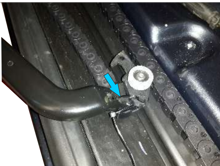
Figure 4. Cancel the lower latch
