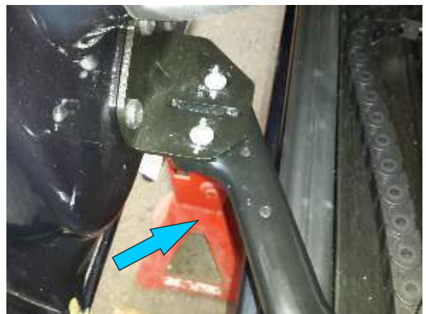
Make marks position lower roller ASSY screws before disassembling
