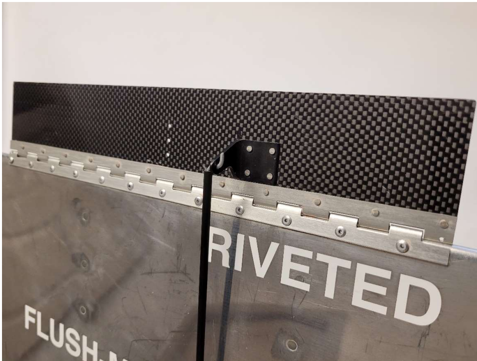
RIVETED INSTALLATION – AILERON BOTTOM VIEW. Trim tab counterweight omitted for clarity.
