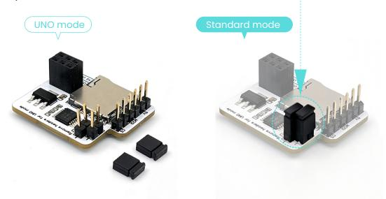
In this mode, the module must be connected to a microcontroller's VCC, GND, and SPI pins.
