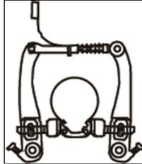
Simply turn the adjusting screw on the brake lever until the gap between the brake shoes and the rim flank averages about 1.5-2 mm.
