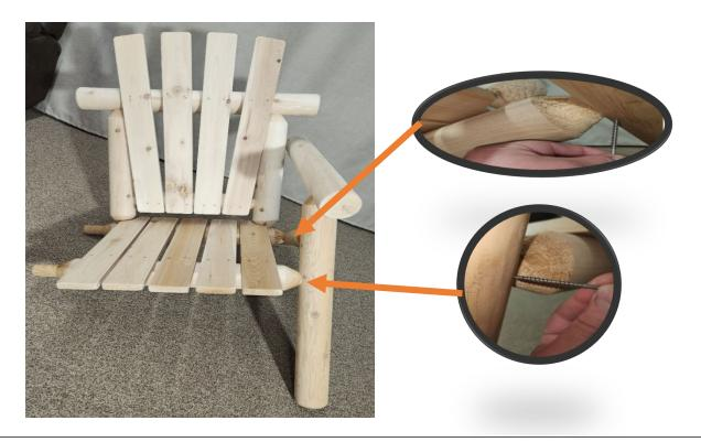
Step 6. Align the predrilled hole in the Arm with the Seat Back Post and put the washer (G) on the  $4 \frac{1}{4}$ " Lag screw (F) and screw it with a  $\frac{1}{2}$ " socket
