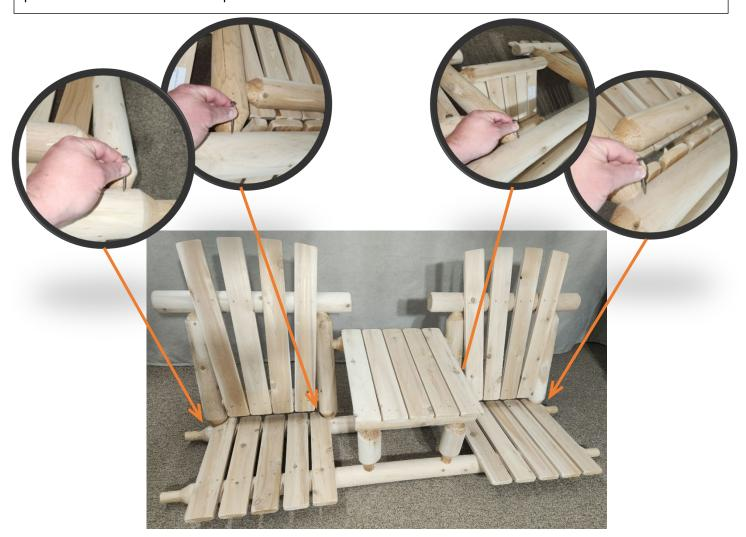
Step 5. Screw (I) screw about ½" behind the side hole of the Chair Back post at a 45° angle so that it hits the Center Table (C) back tenon for both back side tenons
