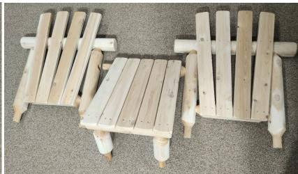
Step 4. Screw (I) screw about ½" below the back of the Chair Back post at a 45° angle so that it hits the Chair Back post tenon for all four Chair Back posts
