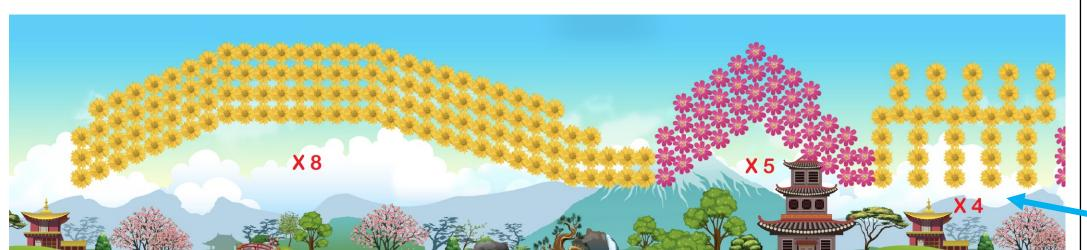
In addition to guiding complex and fully customizable breathing patterns, the Prana Wearable and app can optionally detect and enforce diaphragmatic breathing and upright posture during the breathing exercise training modes. For example, in the visual breath training above, slouching can cause the scrolling to momentarily pause.
