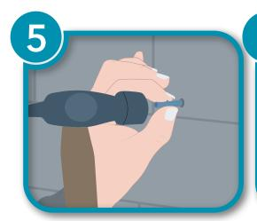
Ensure drilled holes are free of any excess dust and deep enough to accomodate the length of the plugs & screws being used. Gently tap a wall plug into each hole until flush with the surface.
