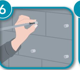
Screw sockets firmly into place x 4. Do not over tighten as you may damage the socket piece. 7 roberts
