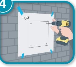
The four points on your template show exactly where you need to drill or screw directly into your wall. (If NOT installing onto masonry go to step 6)
