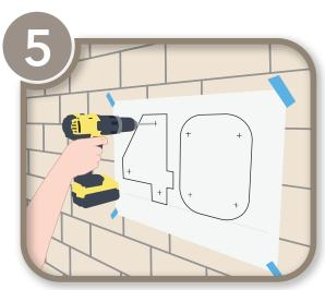
The crossed points on your template show exactly where you need to drill or screw directly into your wall. (If you are NOT installing onto masonry go to step 7)
