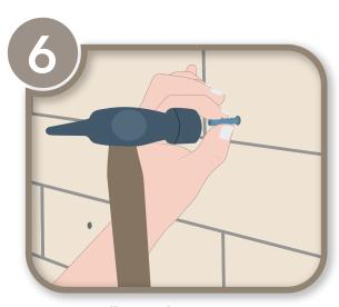
Ensure drilled holes are free of any excess dust and deep enough to accomodate the length of the plugs & screws being used. Gently tap a wall plug into each hole until flush with the surface.
