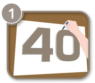
Place your floating numbers on a large piece of paper. Ensure they are level, aligned and spaced exactly as you wish them to be mounted. Trace around the perimeter with a marker pen.
