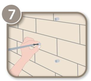
Screw sockets firmly into place. Do not over tighten as you may damage the socket piece.
