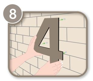
Carefully line up the studs on the back of your floating number with the sockets on the wall and press into place. You will feel a firm click. Visually inspect to ensure all sockets have clicked in.
