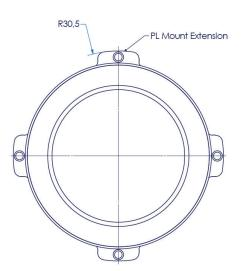
ill. 1: max. measurements of input lens
