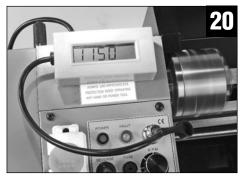
Install/mate the digital readout (optional) to its socket and test operation.
