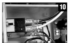
Connect the black and the white wires to the two terminals on the safety switch as shown.
