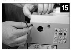
Install gear box cover with 2 screws.
