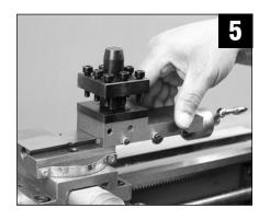
If necessary, re-mount the handle at the rear of the compound rest in the proper position. Then install the compound rest on the cross slide of the carriage. Adjust gibs as required to assemble and for proper operation (See manual for gib adjustment if required).
