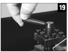
Install all remaining handles, cranks, caps, covers and shields in the locations shown in the assembly diagram.
