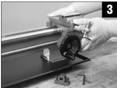
Install the handle and knob to the carriage/saddle apron assembly.
