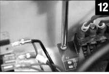
Check all other connections and ensure good contacts. Now, reinstall the circuit board inside the box with the 4 screws previously removed. Note: Screws may not tighten on the board; this is normal. Do not over-tighten.
