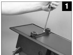
Carefully place the main frame of the machine upside-down on your workbench
