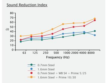
INS have recognised the complex problems associated with noise breakout from ductwork and have developed performance data from laboratory test results.
