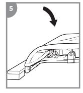
Firmly pull the FRAME out of the RECLINE ADJUSTER by lifting the FRAME with one hand and lift red RECLINE ADJUSTMENT tab up while folding FRAME down flat.
