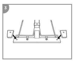
Screw 2 FEET into underside of FRAME with 2 LONG FOOT SCREWS.
