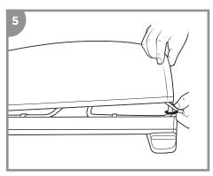
Attach the two black elastic loops on bottom of FABRIC COVER to the chrome STEEL FRAME.
