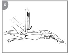
Attach the TOY BAR to the FRAME by pressing clips on to the FRAME
