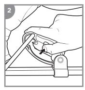
To do this, squeeze the red tab to unlock the RECLINE ADJUSTER.
