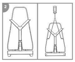
Connect the UPPER FRAME into the LOWER FRAME until tight with UPPER FRAME SCREW holes facing inward.
