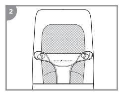
Buckle child into child restraint and secure buckles through either slot on each side (depending on size of child).
