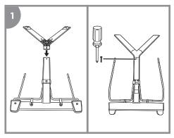
Connect FRONT BASE FRAME to BACK BASE FRAME with BOLT on the underside of the frame.
