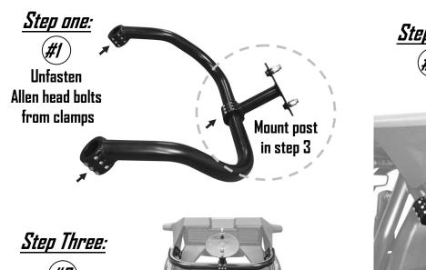
Center, mount and position wheel post. Position Dual clamp evenly on to roll cage, above shock reservoirs.
