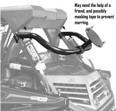
Angle wheel post to where tire rubber rests on the cross bar when fastened.
