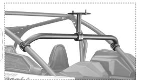
Intrusion bars Unfasten all Allen Clamp Bolts, loosely fasten one side at a time.
