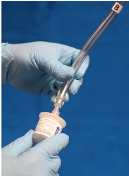
Figure 5: Hose B connection with Test Filter
