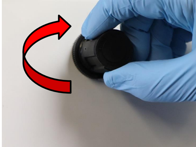
Figure 11: Turning Pressure regulator to allow airflow in the system
