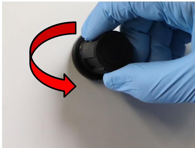
Figure 8: Turning Pressure regulator to stop airflow in the system
