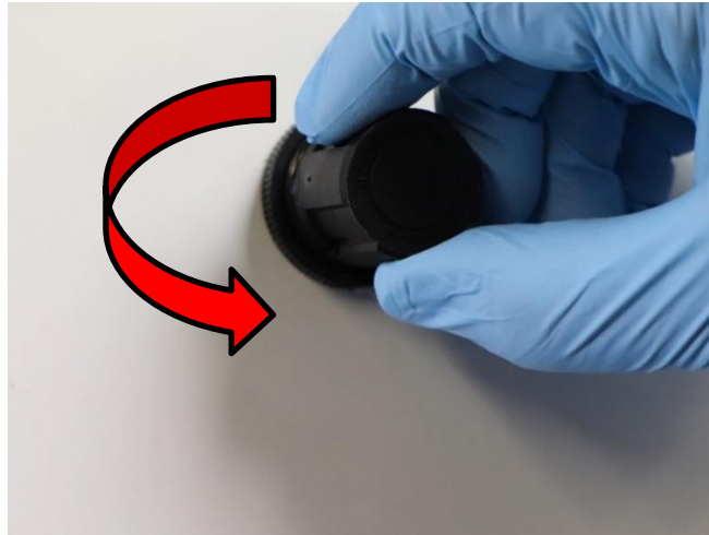
Figure 12: Turning Pressure regulator to stop airflow in the system
