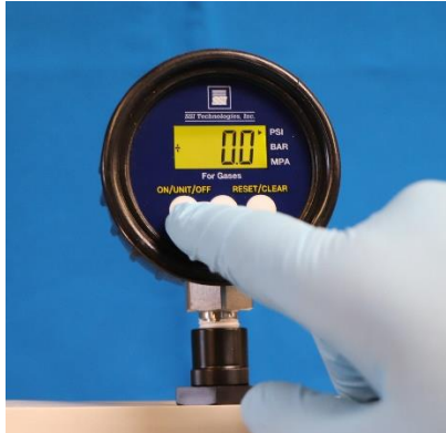
Figure 7: Switched on pressure gauge with lit screen
