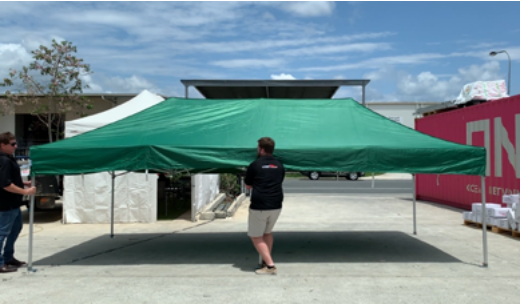
9. Middle Legs. Lift the front back roof connectors until pins locks in to position.
