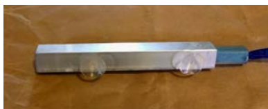
Figure 2: Optional heater in the bottom of the inner bucket
